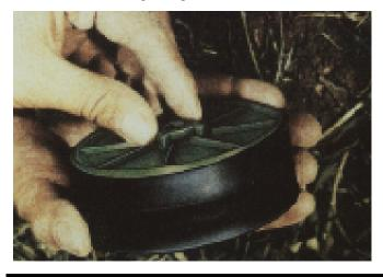
$\underline{\rm Figure~No.~1}.$  Typical Anti-personnel mine manufactured in the former Yugoslavia and Deployed in Bosnia.
